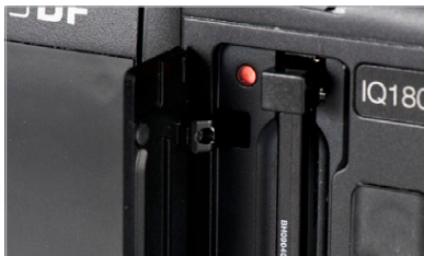
Installing and removing the CF card
